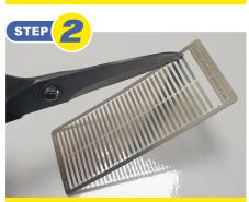
Carefully **cut the Track Power Boosters** from the sprue using your sharp scissors. Don't be tempted to wiggle the part back and forth in order to break the joint as you may bend or distort the Booster which will make it difficult to put into place later.
